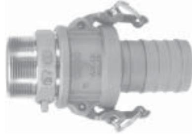
The Cast-in lugs allow safety clips to be attached once the lugs are passed through slots in the special cam lever arms. These clips prevent the coupler from being unlocked until they are removed, providing a **positive locking action.**
